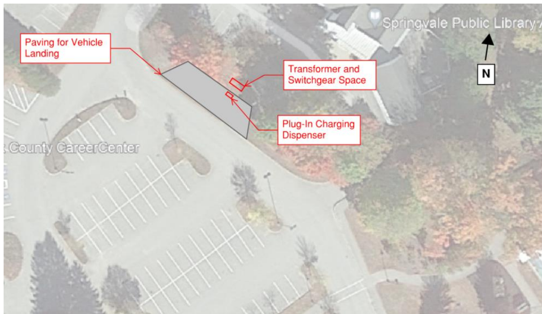
Figure 17 Conceptual Layout of Charger at the Nasson Healthcare Site (Source: Google Earth)
